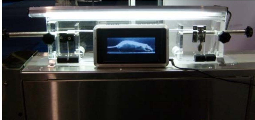
Figure 1.4 DigiGait™ made by Mouse Specifics Inc. The system has a treadmill on the bottom of the transparent compartment. The speed of the treadmill and the size of the compartment are adjustable. A video camera records bottom images of the rat that walks through the system. All the locomotion parameters are generated from the analysis of the images.
