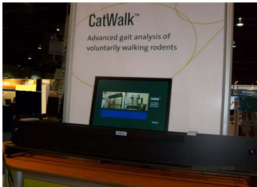
Figure 1.5 CatWalk™ invented by Noldus Information Technology. The floor of the system is transparent and lightened by arrays of LED. Only at the points where a paw touches the glass, light exits the floor and scatters at the paw, illuminating the points of contact only (Noldus IT, 2006).
